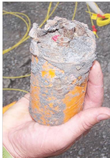
Examples of boosters that have been loaded into wet holes showing the impact of water.
