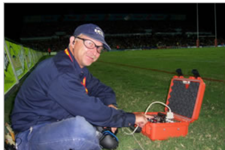
Electrical firing isolates operator from normal and malfunctioning fireworks blast, heat, projections and noise.
