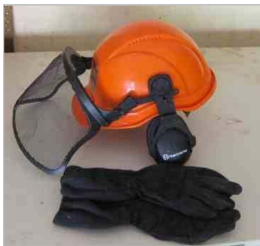
Hand firing requires additional PPE
